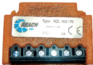
6선 전파 정류기, 수직 설치형 6-Wire Full-Wave Rectifier, Horizontally Mounted
